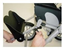
Put the back insert into the back base of the backrest and adjust to the desired height by tightening the clamping bolts. If your BINGO is delivered with a canopy accessory, put the adapter fittings on the tubes with the back insert in place. Refer to chapter 5 accessories 5.17 canopy.
