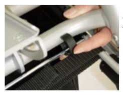
The storage bag is attached with clips to the cross member of the front frame and with snap fasteners to the rear frame.
