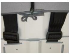
Fix the shoulder straps to the slots in the back base as described in 5.5 lap belt
