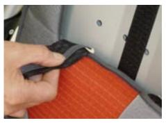
Lead the shoulder straps together with the pad straps through the designated slots in the back insert
