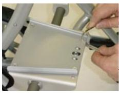
Before use in the reverse riding direction the base adapter must be rotated 180°.
