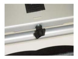
Insert the abduction block with its flat link through the slot in the front part of the seat upholstery into the designated rectangular slots (upper and lower!) in the very front of the seat plate. Clamp the abduction block by turning the wing nut of the clamping set.
