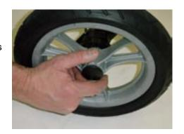
To attach the wheel push it onto the axle until the quickrelease snaps in automatically.
