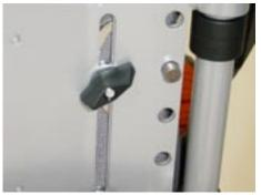
After loosening the wing nut the trunk pad width can be adjusted by swinging the crank from horizontal to vertical.
