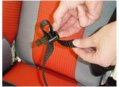
Then thread the tensioning straps into the buckles.
