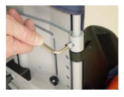
From a back height of approximately 55 cm for seat size 1 and 66 cm for seat size 2 the back frame has to be placed to the lower position on the back metal sheet.
