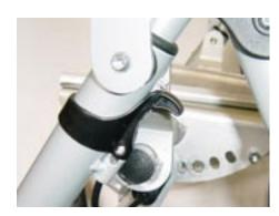
• Swing the knee angle assembly with the footrest to the desired position and fix it with the clamping lever
