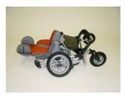
After disengaging the folding guards hold the upper part of the push handle and fold it forward until it touches the front frame and the pushchair is lying on the floor
