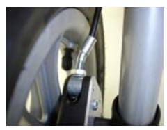
At the exit of each brake housing a cranked set screw leads the brake cable away from the tire of the rear wheel. After loosening the counter nut the pre tension of the individual (left or right) brake can be adjusted.
