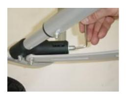
Make sure that the suspension is adjusted equally on both sides. The scale in the window of the spring housing offers an orientation.
